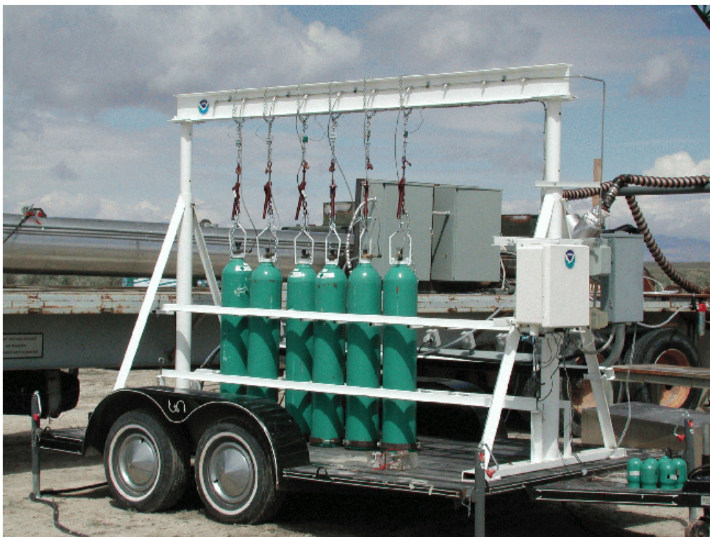
Figure 2. Mobile SF 6 release mechanism showing SF 6 bottles suspended from load cells in the white bottle rack. The mass flow controller and data logger are in the back of a 3/4 ton van that is parked next to the rack during active tracer releases. The mobile DPG stack is in the background.
