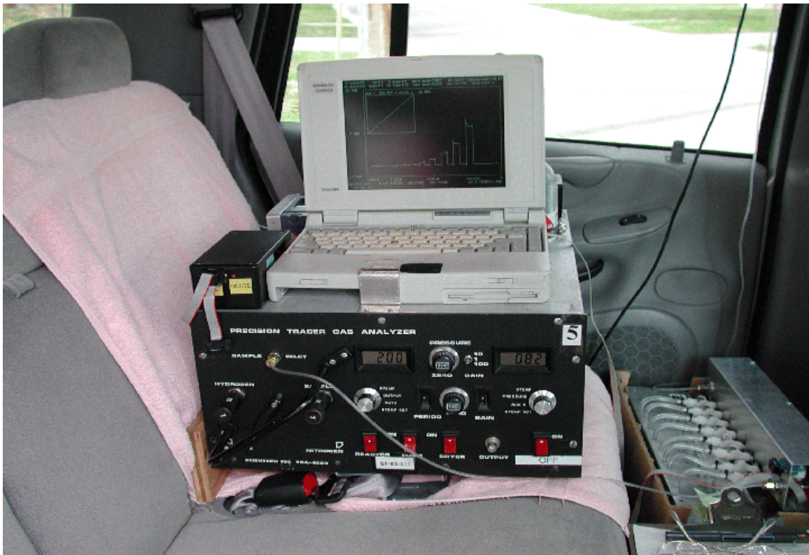
Figure 4. NOAA continuous mobile SF 6 tracer gas analysis system installed in the rear seat of an SUV, showing computer controlled TGA-4000 (bottom) and calibration gas container (lower right).
