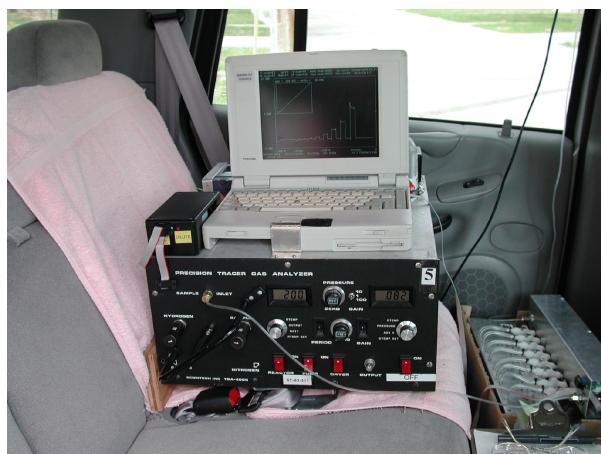
Figure 2. FRD continuous mobile SF 6 tracer gas analysis system installed in the rear seat of an SUV, showing computer controlled TGA-4000 (bottom) and calibration gas container (lower right).
