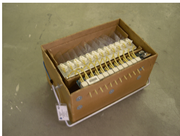
Figure 4. Time-integrated SF 6 bag sampler with installed 12-bag cartridge. D-cell battery is shown in lower-right.
